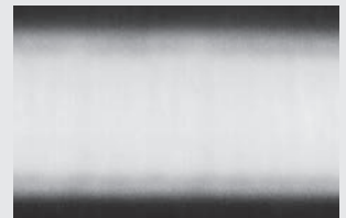
Latex paint through a HEA 517 tip at 10,000 psi
