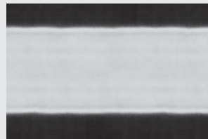
Latex paint through a standard 517 tip at 10,000 psi
